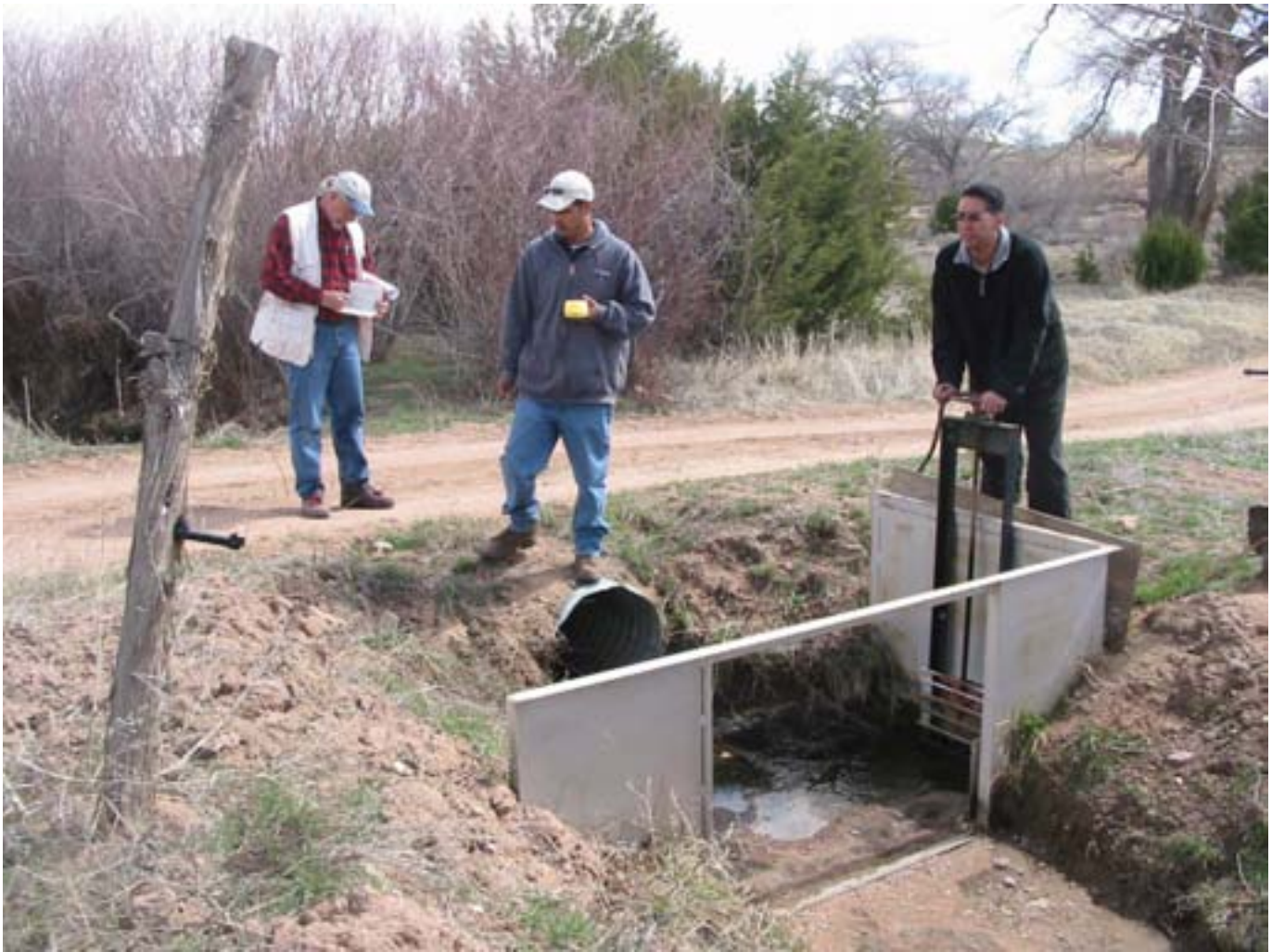
Figure 4. GPS Technicians acquiring GPS data at diversion structure
